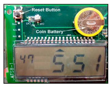
Figure 6-9. Reset Button Location.
